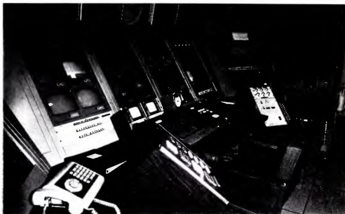
Master control console is a Norelco design with CDL 17-event memory control unit.
