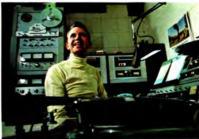
Closer shot of second studio shows Gates console, on control desk at right, open-reel and cart tape machines on rear wall. Door to news room is at left rear.
